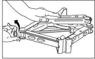
You will need to turn the plastic wheel nut counterclockwise to loosen the wheel wrench from the jack.
