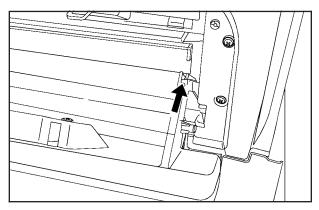
Release the glove box stops by pushing them both outward to let the glove box drop open completely.
