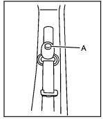
To move it down, press the release button (A) and move the height adjuster to the desired position. You can move the height adjuster up just by pushing up on the shoulder belt guide.
