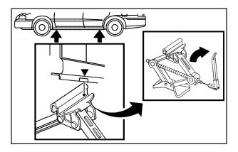
Position the jack and raise the jack lift head to fit over the car flange under the down arrow markings on the rocker panel.
