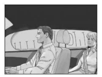
If your vehicle has a side impact airbag for the right front passenger and the person directly behind that passenger, it is located in the ceiling above the side windows.
