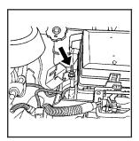
The remote positive terminal is located under a red tethered cap on the engine compartment fuse block. Remove the cap to access the terminal.
