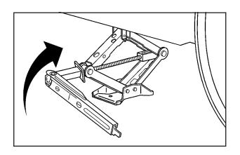
Raise the vehicle by turning the jack handle clockwise. Raise the vehicle far enough off the ground so there is enough room for the compact spare tire to fit underneath the wheel well.
