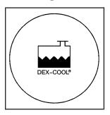
The coolant recovery tank cap has this symbol on it. The tank is located in the engine compartment toward the front of the engine on the passenger's side of the vehicle.
