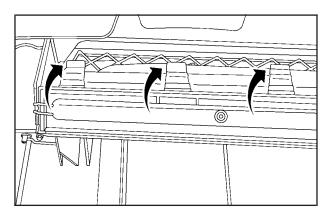
Pull each of the three tabs of the filter access door down and open the access door downward.
