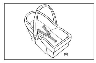
An infant car bed (A), a special bed made for use in a motor vehicle, is an infant restraint system designed to restrain or position a child on a continuous flat surface. Make sure that the infant's head rests toward the center of the vehicle.
