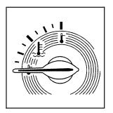
Your vehicle has an engine coolant temperature gage. With the ignition turned to ON, this gage shows the engine coolant temperature.
