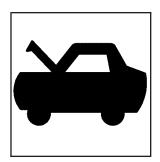
Pull the interior hood release lever with this symbol on it. It is located to the left of the instrument panel on the driver's side of the vehicle.
