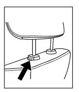
Pull up on the head restraint to raise it. Press the button at the base of the head restraint and push the head restraint down to lower it. Only the front head restraints are adjustable.
