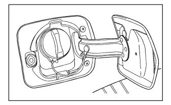
The tethered fuel cap is located behind a hinged fuel door on the passenger's side of the vehicle.
