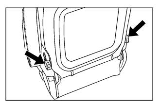
3. Use one of two levers to fold the seat flat. The levers are located on the rear of the seat near the bottom of either side of the seat. Pull up on either lever and fold the seat forward until the seatback disengages. This can most easily be down from the rear seats.
