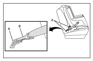
Lower anchors (A) are metal bars built into the vehicle. There are two lower anchors for each LATCH seating position that will accommodate a child restraint with lower attachments (B).
