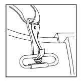
5. Attach the strap to the cargo tie-downs in the rear of the vehicle.
