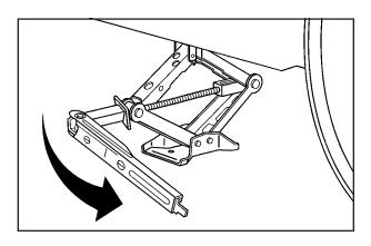
Lower the vehicle by turning the jack handle counterclockwise. Lower the jack completely.
