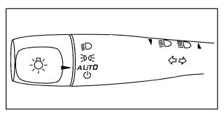
The lever on the left side of the steering column operates the exterior lamps.
