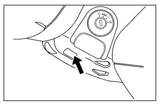
2. Using a tool, pry off the cover from the bottom of the steering column.
