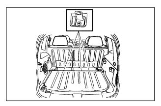
The top tether anchors are located in a storage compartment behind the rear seats. Lift the lid of the storage compartment to access the anchors. Be sure to use an anchor located on the same side of the vehicle as the seating position where the child restraint will be placed.
